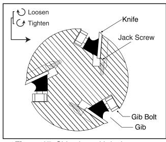
Figure 17. Side view with jack screws.
